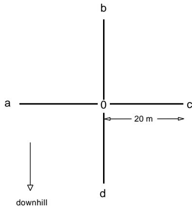
Figure 1. Field sampling layout. At each site four 20-m transects were sampled: from point a to the center (data file labeled a0), from the center to point c (0c), from point d to the center (d0) and from the center to point b (0b).
